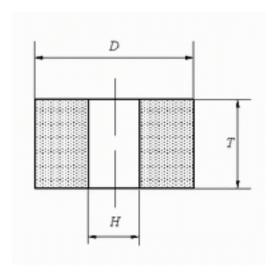
Small plain wheels (Small Wheels) Code 1A8(PX) Binder B.M(S.Q)
